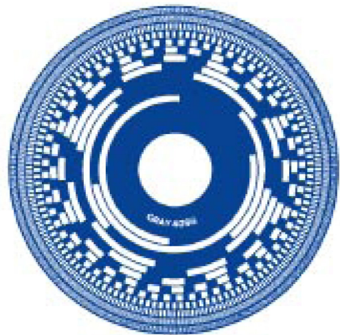
Figure 3: Code disc for an optical absolute encoder features one track for each bit of resolution. The number of bits n ( 2^n ) corresponds to 2^n radial positions.
